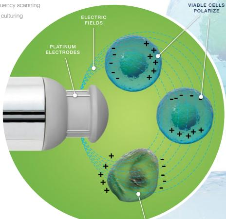
DEAD CELLS HAVE DAMAGED MEMBRANES AND DO NOT POLARIZE
